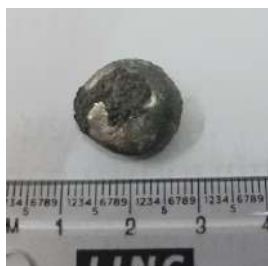
Plasma arc furnace Iron metal
