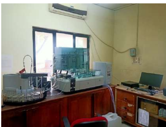
Figure 3. Continuous Flow Analyser for simultaneous multi-parameter analysis
