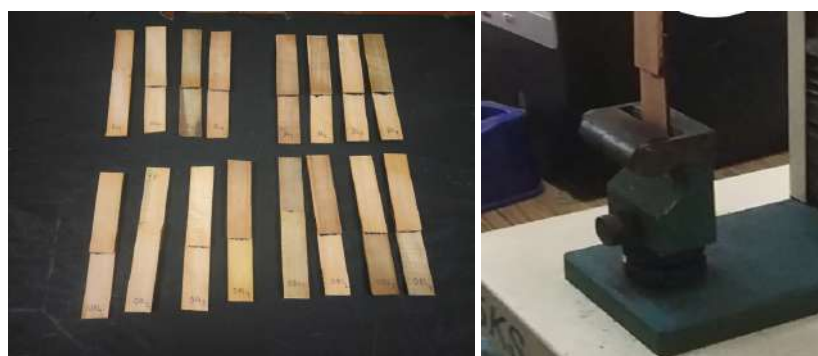
Fig. 51. Mechanical testing of formulated lignin-glyoxal adhesive by lap shear method.
