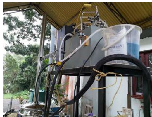
Figure 7. Photograph of incinerator prototype unit
