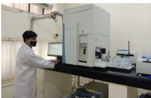
Figure 5. Inductively Coupled Plasma Mass Spectrometer (ICPMS) Facility
