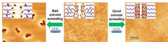
Atomic force microscopy images of block copolymer supramolecules before (middle) and after annealing in good and bad solvent vapors. Schematic illustrations of the hierarchical assembly of small molecules within the block copolymer microdomains are shown in the insets.
