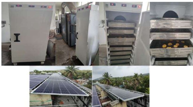
Integrated rooftop model for solar dehumidified driers
