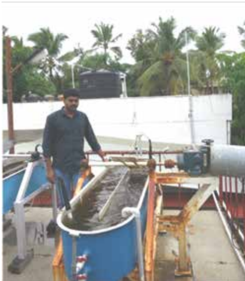
Figure 6. Outdoor 1m 2 area seawater raceway pond with brown algae. The pond is dark brown and measured light absorption exceeds 90%.
