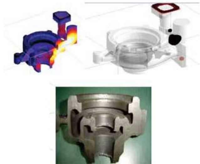
Figure 20. Shrinkage defects as predicted by AutoCAST XI for two industrial castings
